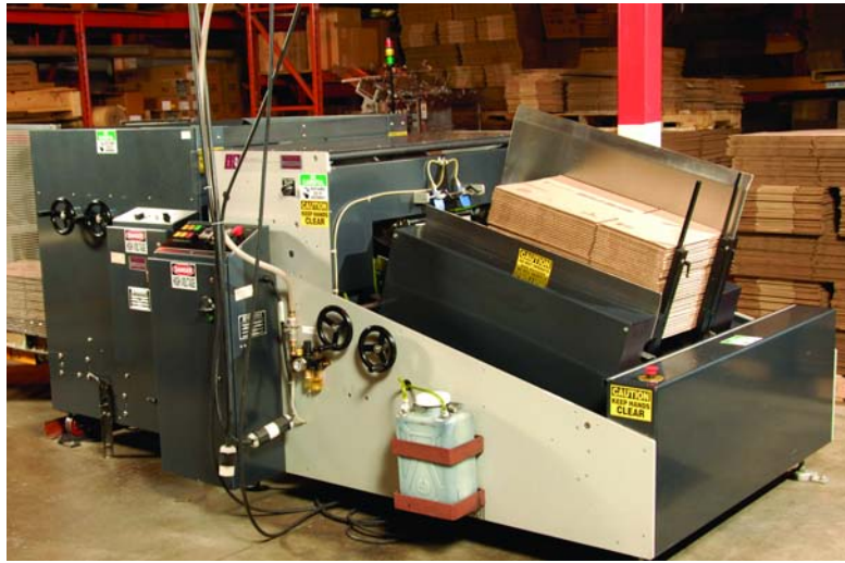
Bundles of printed cases sit in the feed magazine of the Optimizer off-line digital case printing system at the Burlington production facility.
