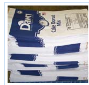
Bundled bags with 9 × 8-in. printed ingredient statement are stacked onto a pallet in alternating layers for stability.
