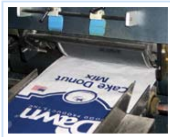
Baking bag engaging with the Maximizer print cylinder.
