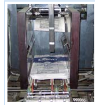
Baking bag with 9 x 8-in. printed ingredient statement comes off the print cylinder and is bundled in the restacker for ejection onto the conveyor.
