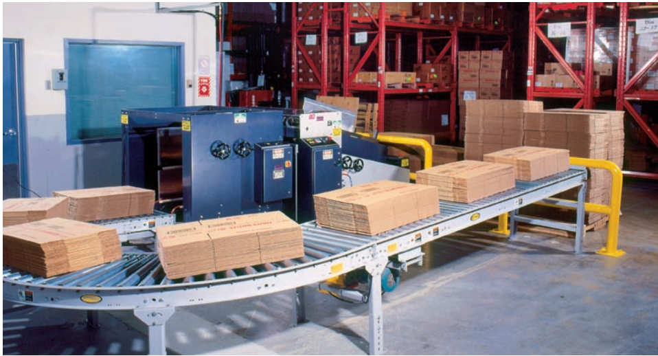
Coded cases, in stacks of 25, move along a powered roller conveyor and are stored for later use.
