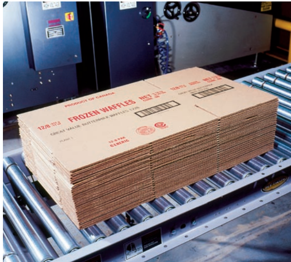
A stack of coded cases moves along a conveyor, left. The digital case printer produces in-spec bar codes at a 200-dpi resolution. A restacker, right, restacks coded cases as they are completed.
